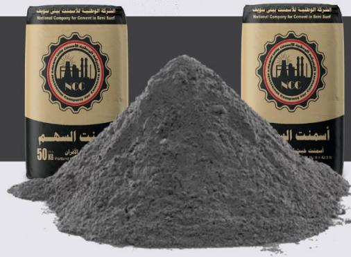
Blast furnace Cement - Low stress resistance in early days and outperforms all types of cement in the late days. Resistant to sulfate and chloride salts.
